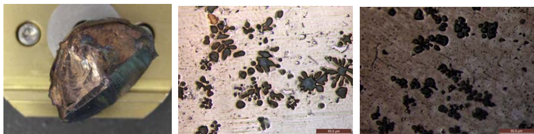
Fig 6. Ingot and microstructure of U-Mo-1.0%O
